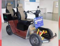
Seat Leg Space:400/380 MM Steering Mech: Ackerman Wheel Diameter: 500 MM
